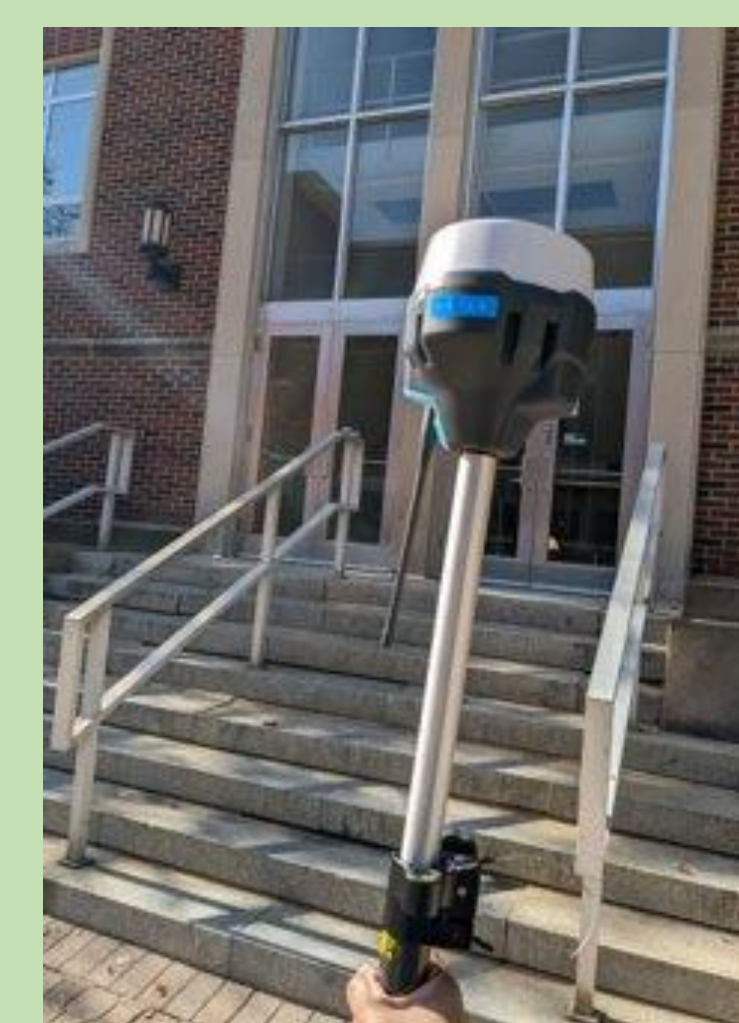
Figure 3. Survey-grade GNSS units can be used as a reference for determining accuracy
